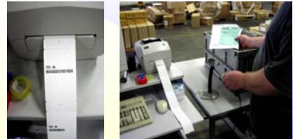
Printing NVE Label with integrated RFID Transponder PLUS writing on RFID Chip
